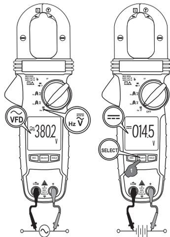
**Note :** **ACV**(and hence **Line-level Hz**) function is equipped with digital low-pass filter, & is capable of dealing with **VFD** (Variable Frequency Drive) signals. It also improves ACV reading stability in noisy electrical environments.
