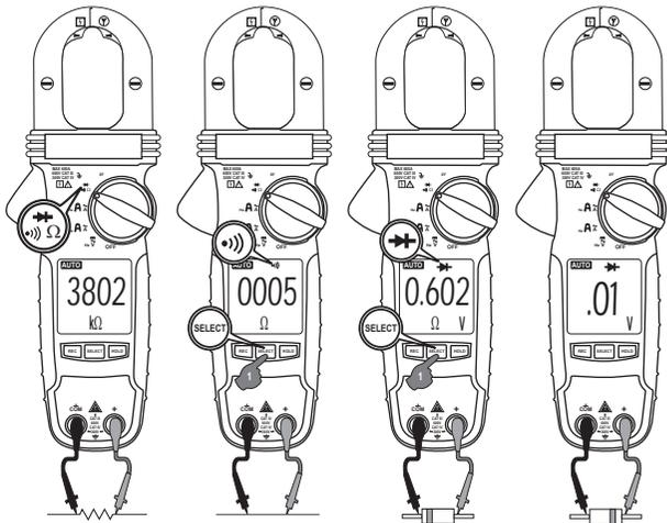
**Note :** When using diode test function, normal forward voltage drop (forward biased) for a good silicon diode is between 0.400V to 0.900V. A reading higher than that indicates a leaky diode (defective). A zero reading indicates a shorted diode (defective). An OL indicates an open diode (defective). Reverse the test leads connections (reverse biased) across the diode. The digital display shows OL if the diode is good. Any other readings indicate the diode is resistive or shorted (defective).
