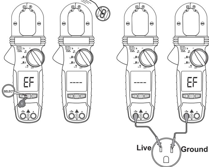
❖ **Non-Contact EF-Detection** : An antenna is located along the top-right end of the stationary clamp jaw, which detects electric field that surround energized conductors. It is ideal for tracing live wiring connections, locating wiring breakage and to distinguish between live or earth connections.
